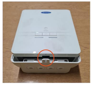
Remove Genesis control panel cover by pushing the cover up.
