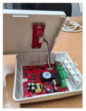
Once the case can be lifted, carefully remove the wiring from the cover of the control board.
